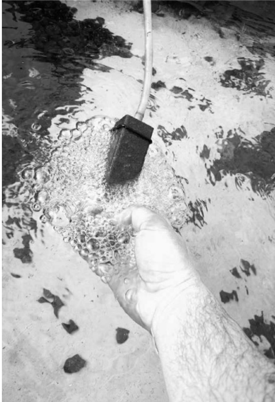
Air stone actively aerating the water. Notice the O-ring bumper.
