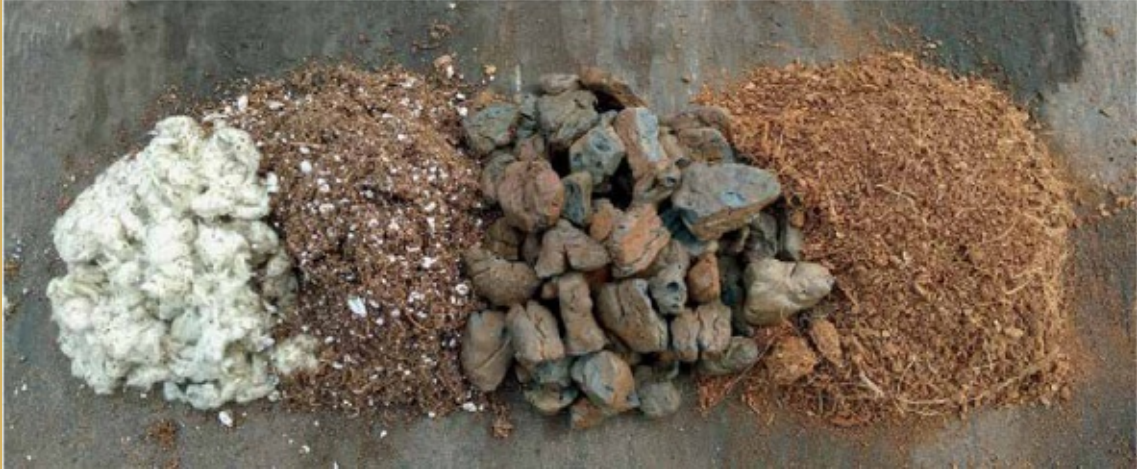
Substrates from left to right: loose rockwool, Pro-Mix, expanded clay pebbles, coco coir.
