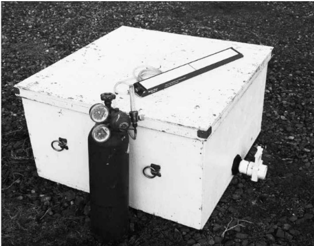
Live haul setup: fish transport tank, oxygen tank, pressure regulator, flow meter and micro-bubble diffuser.
