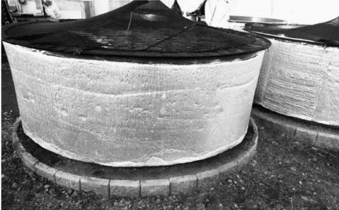
Insulated fish tanks.
