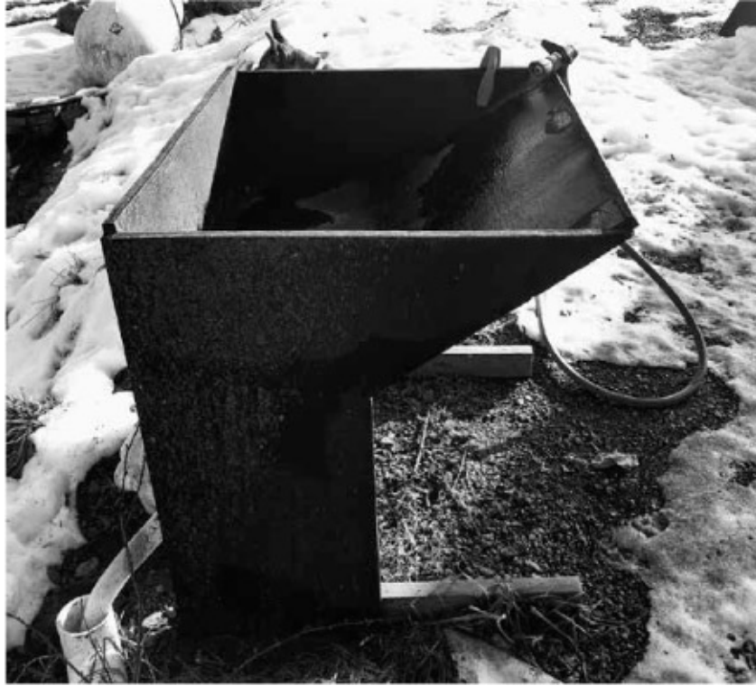
Our wash down sink, constructed of plywood and coated with liquid rubber, plumbed into the Waste Tank.
