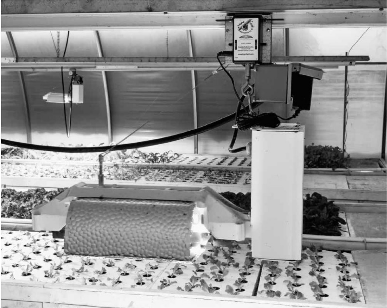
Gavita Pro 1000-DE on a LightRail mover.
