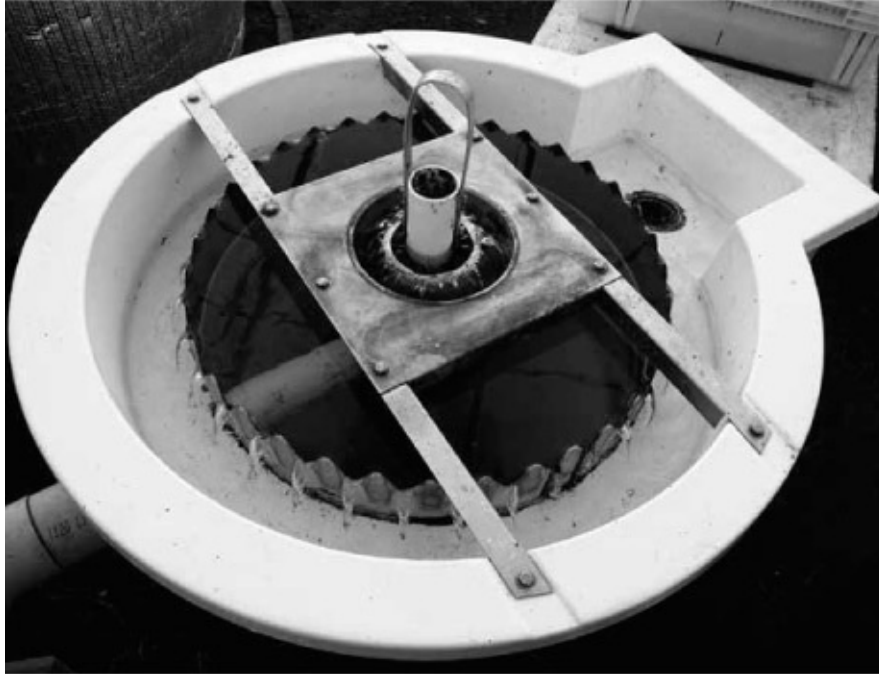
Top of the RFS, showing the stilling chamber and the overflow weir.
